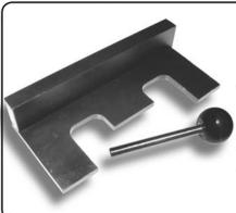
Needed for the crucial task of aligning the cam shaft with the Bosch Diesel injection pump. This two piece lock plate and alignment pin allows the technician for factory correct and trouble free installations every time.
