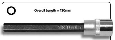
This special LONG 8mm Hex Socket with a 1/2" drive, was designed with the extra reach needed for proper clearance to R&R head bolts. Applicable: Mercedes engines - M115, M116, M117.
